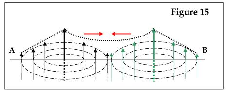
The contrary happens if the two electrical currents have opposite direction, for the velocities induced in the plenum between them subtract from each other, which results in a local slowing down of the flux of plenum. In this case, the circulations of the velocity field invert their algebraic signs with respect to the former case, and the action between the two electrical current lines becomes repulsive.
