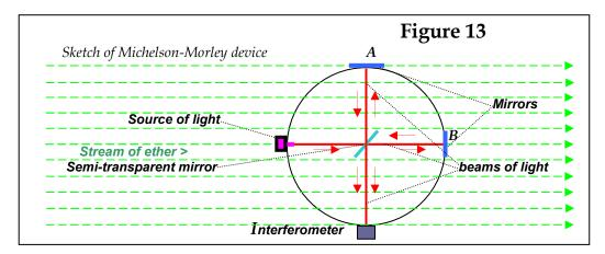
In Michelson's view, the two mutually orthogonal beams reflected by mirrors *A* and *B* should travel across the stream of ether according to different speeds with respect to the observer (the interferometer in the figure above), thus generating interference fringes.
