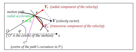
The figure above is the representation of a point that moves along any plane path, at a variable velocity  $\vec{V}$  expressed through the relevant vector notation:
